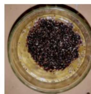
Figure 8. F5 bio-adsorbent, after 4 hours contact time
