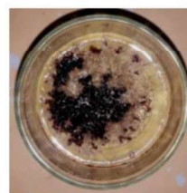
Figure 4. F1 bio-adsorbent, after 4 hours contact time
