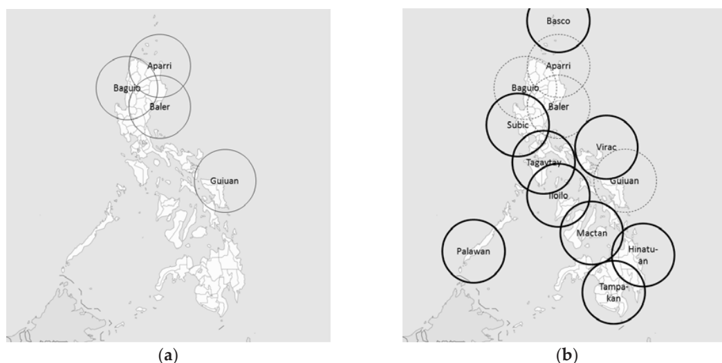
Figure 5. Comparison of Doppler radar distribution nationwide in 2010 versus 2015: (a) location and coverage of functional Doppler radar facilities in June 2010; (b) location and coverage of functional Doppler radars by the end of 2015. Data source: PAGASA.
