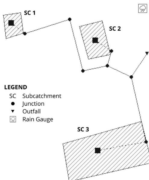
**Figure 3.** SWMM model of the three subcatchments in DLSU – Laguna Campus
