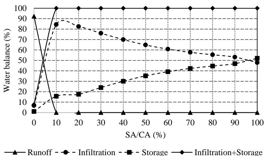
**Figure 7.** Water balance elements with respect to SA/CA ratio at 80<sup>th</sup> percentile rainfall
