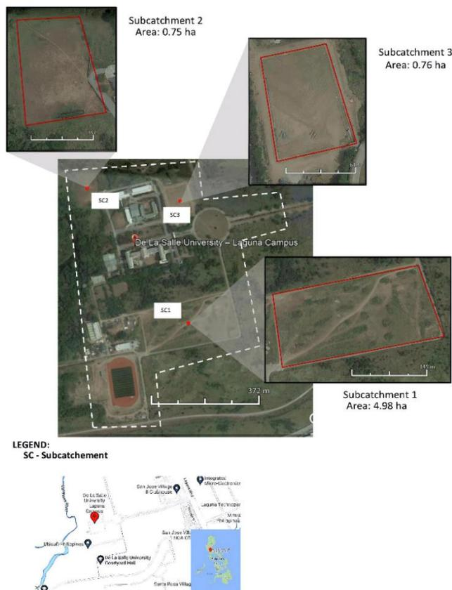
**Figure 1.** Site map displaying a satellite view of the DLSU – Laguna Campus with the chosen subcatchment areas highlighted and their corresponding areas indicated.
