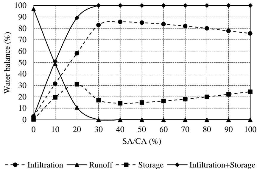
**Figure 8.** Water balance elements with respect to SA/CA ratio at 90% percentile rainfall
