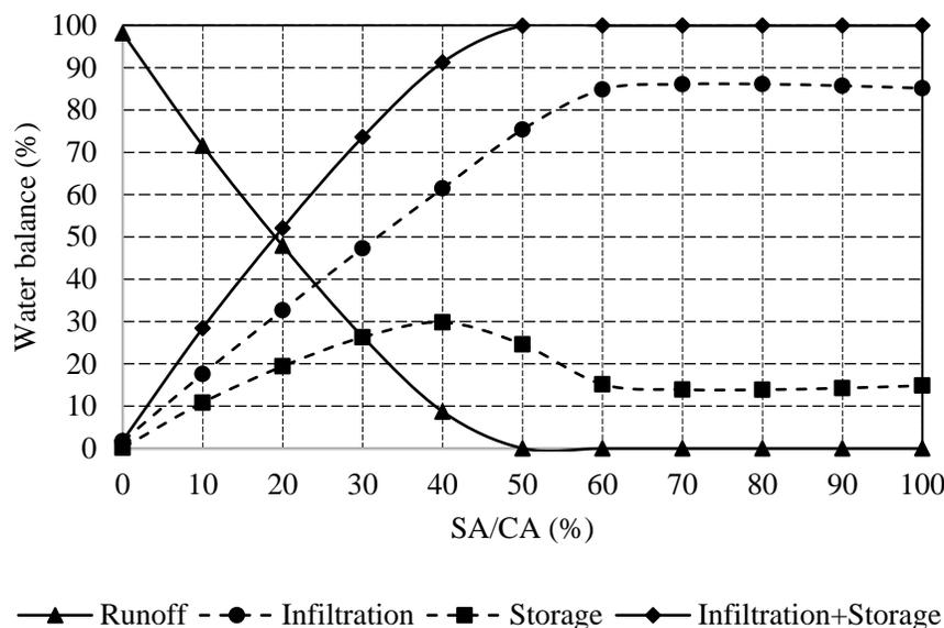
**Figure 9.** Water balance elements with respect to SA/CA ratio at 95<sup>th</sup> percentile rainfall
